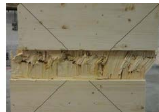
Shear perpendicular to the grain
